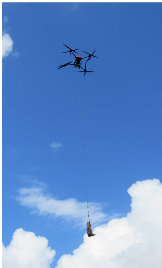
Figure 3 Shows a DJI T40 Agras drone carrying a hessian sandbag containing approximately 15kg of mangos on a ten-metre rope. This method allows the drone to be continually seen, visual line of sight, while lowering the payload to the ground below a low tree line.
